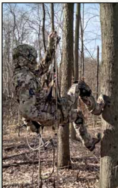
The right hand controls speed of descent. The left hand opens the brake handle. Always use both hands!
