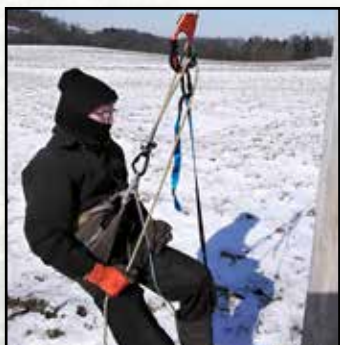
Notice the correct shortened bridge length. Foot loop is clipped to the ascender. Safeguard is connected to saddle.
