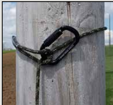
Pull down to lock. If done properly it should stay in place when load is removed.
