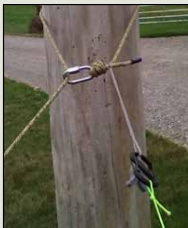
After descending, pulling the loop away from the tree will open the loop. Pull until end is completely free.
