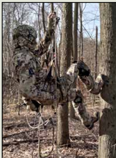
The right hand controls speed of descent. The left hand opens the brake handle. Always use both hands!
