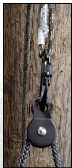
Pulley used for a friction free bridge pivot
