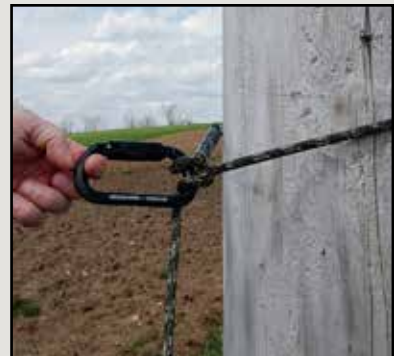
Pulling sideways will easily open the loop, allowing quick and secure position changes. Push carabiner in while pulling on main line to relock.
