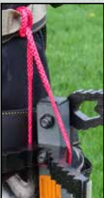
8" loop used to attach a stick to your saddle as you climb.
